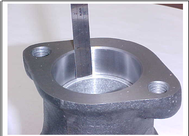
Figure 25 - Seated Piston Depth.
